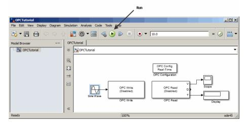
The model writes a sine wave to the OPC server, reads back from the server, and displays the wave in the scope trace. In addition, the quality value is set to 192, which indicates a good quality (see "OPC Quality" on page A-2).
