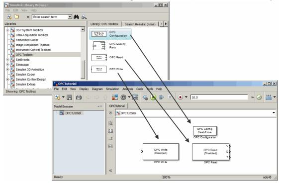
**Note** Block names are not shown by default in the model. To display the hidden block names while working in the model, select **Display** and clear the **Hide Automatic Names** check box.
