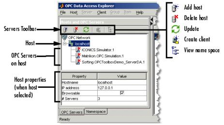
Note that the local host in this example provides three OPC servers. The Server ID for this example is 'Matrikon.OPC.Simulation.1'.
