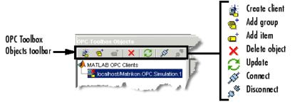
Click **Connect** in the **OPC Toolbox Objects** toolbar. If the client is able to connect to the server, the icon for that client in the **OPC Toolbox Objects** tree will change to show that the client is connected. If the client could not connect to the server, an error dialog will show any error message returned. See "Troubleshooting" on page 1-21 for information on why a client may not be able to connect to a server.
