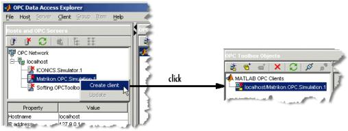
The name of the client (displayed in the **OPC Toolbox Objects** pane) is *Host/ ServerID*, where *Host* is the hostname and *ServerID* is the Server ID associated with that client. In this example, the client's name is 'localhost/ Matrikon.OPC.Simulation.1'
